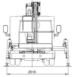
Beams retracted in shape
